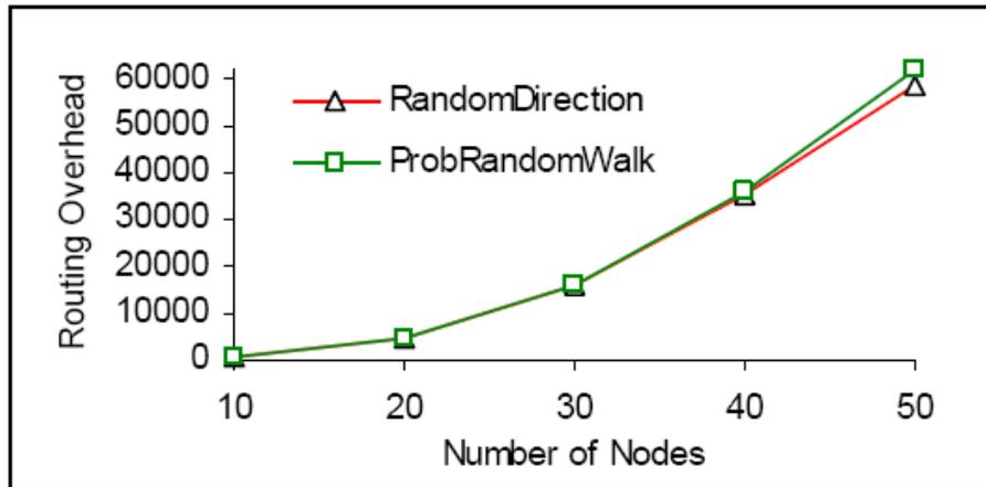
The total number of routing packets also counted per hop. As shown in figure 4 Routing Overhead is more in the Probabilistic random walk mobility model as it increases with the number of nodes. So we analyze the result that random direction gives the better performance under the routing protocol AODV and Routing Overhead is more in Probabilistic Random Walk.
